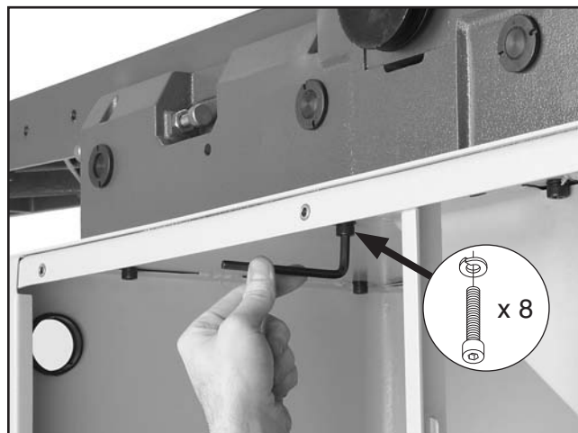
Figure 11. Securing the jointer assembly to the stand.
